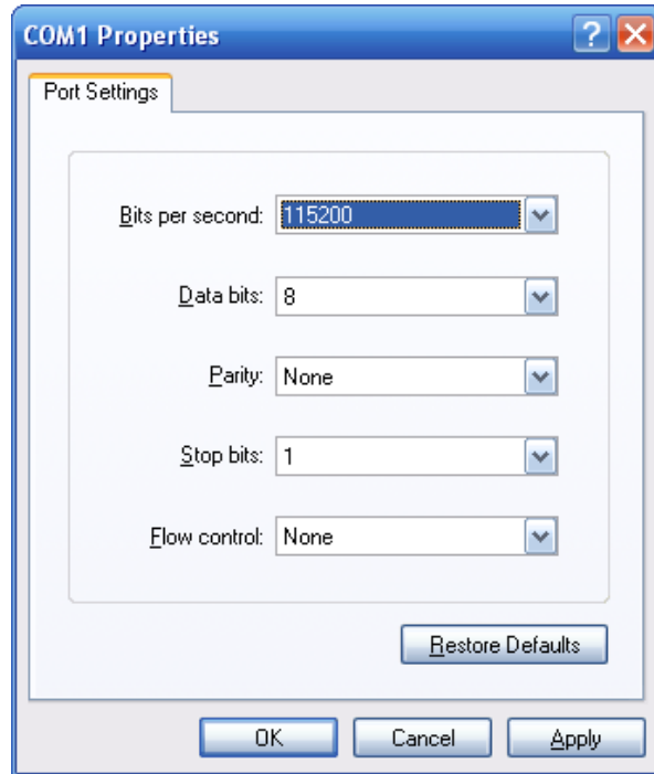
Figure 2-3 Hyper Terminal COM Port Configuration
